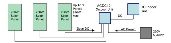
Like all DC-Inverter air conditioners, the ACDC12 compressor runs on DC power converted from AC power. But this special solar air conditioner can also accept DC power directly from solar panels, without needing an inverter, controller, or batteries. The solar DC power directly replaces an equivalent amount of AC power from the power company and can cut daytime energy costs for air conditioning or heating by up to 80-90%.
