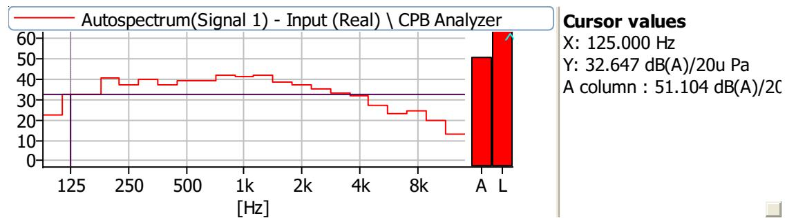
The red line in below curve is 15K noise data. It is within the NC40 level.
